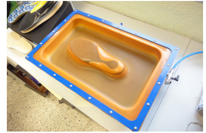
3. Mould the orthotic until it is hard
